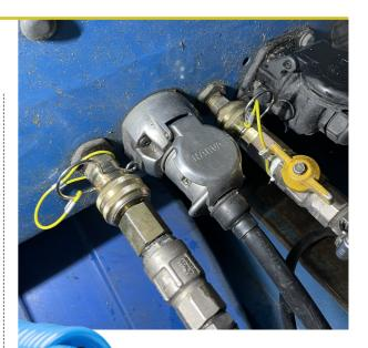
PICTURED: GP Truck Products' CLIPLOCK is designed to improve the connection of airlines and prevent unintentional decoupling. Image: General Pneumatics
